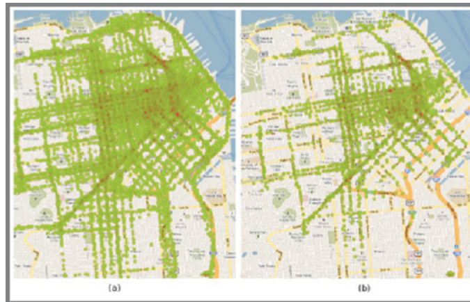
Figure 6 High Density vs Low Density Wi-Fi AP Coverage
